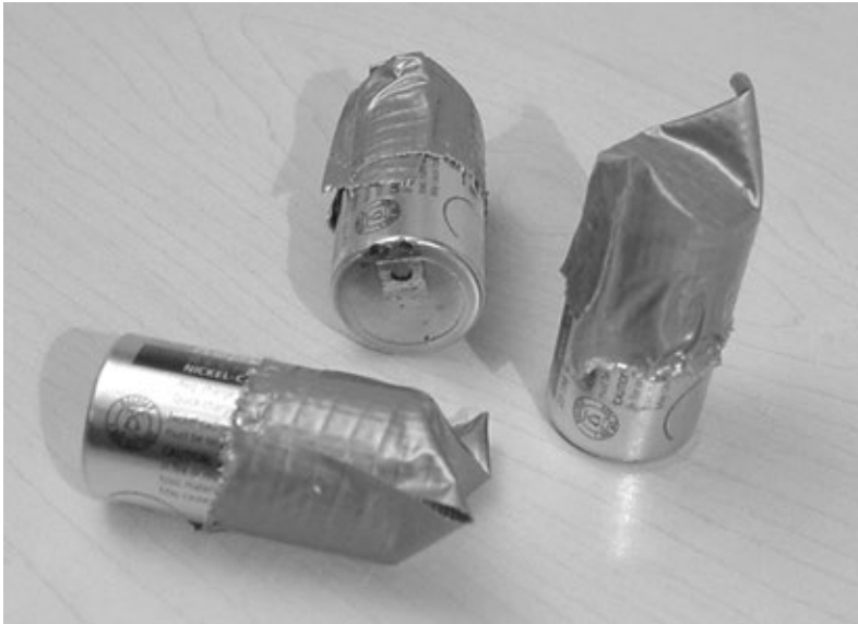
FIGURE 9-9 NiCd cells with taped ends.
