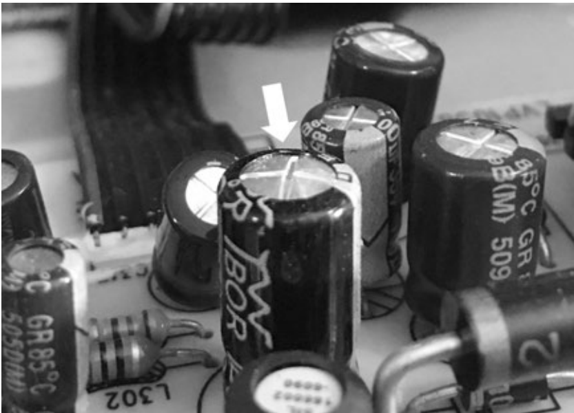
FIGURE 8-14 Bulging electrolytic capacitor.
